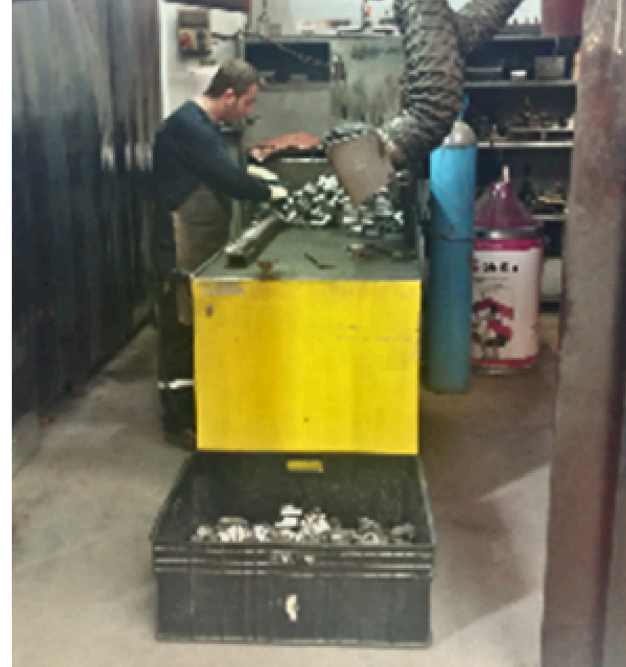
GAZALTI KAYNAK TEZGAHI 1.2 mm Tel / 320-500 A ARCTECH (3 adet) GEDİK FRONIUS (1 adet) EXPRESS WELD (1 adet) TURALLAR (2 adet) DAIHEN (1 adet)
