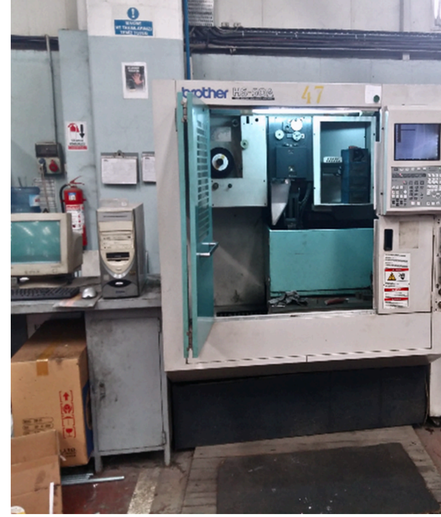
BROTHER HS-50A 4 Eksen Tel Erozyon Tezgahı (x:420/y:260/z:160)
