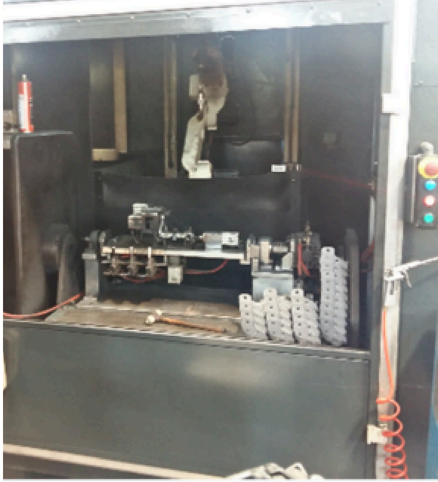
GAZ ALTI KAYNAK ROBOTO 350 A DAIHEN (1 Adet)
