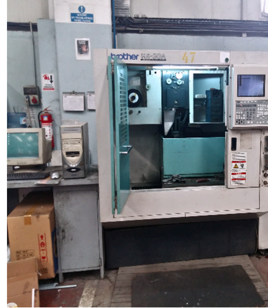
BROTHER HS-50A 4 Axis Wire EDM Machine (x:420/y:260/z:160)
