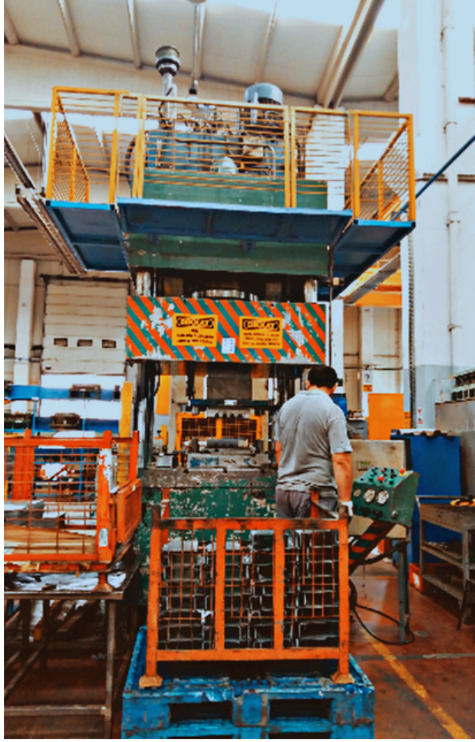
HYDRAULIC PRESS CEMTAŞ 400 TON (1200 X 1600 1200 X 1600)
