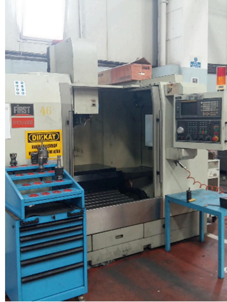
FIRST MCV 1000 3 Axis CNC Machine (x:1000/y:500/z:500)
