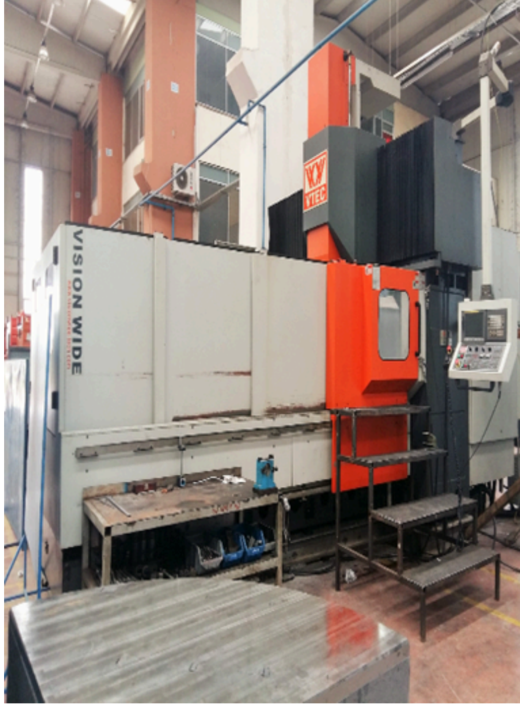
VTEC 3 Axis Bridge Type CNC Machine (x:2450/y:3450/z:900)
