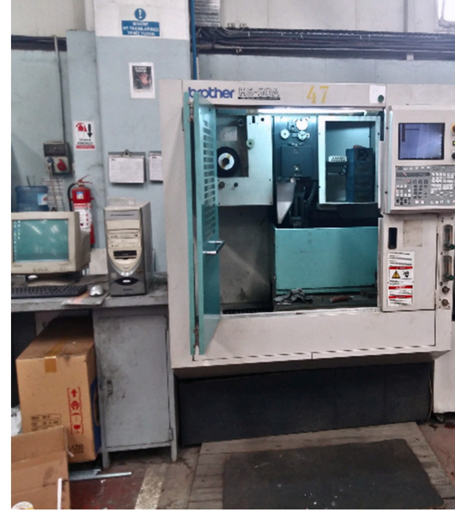
BROTHER HS-50A 4 Eksen Tel Erozyon Tezgahı (x:420/y:260/z:160)
